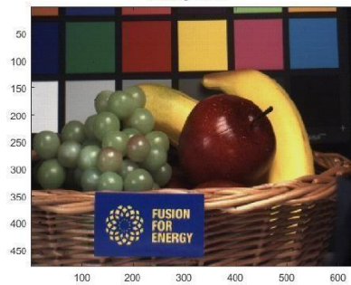
Image captured with a FURHI VGA chip exposed to 1 MGy(SiO 2 ), 10 keV X-ray ON
